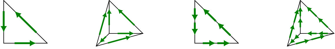
Figure 5.4.: Lowest order Nédélec elements of first and second kind for triangle and tetrahedron.
