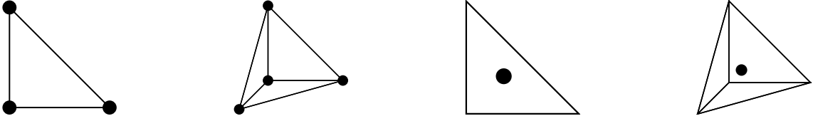
Figure 5.2.: Lowest order H^1 - and L^2 -conforming finite elements for triangle and tetrahedron.
