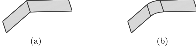
Figure 7.9.: Construction of approximation of discrete jump in 3D. (a) The affine curve with junction. (b) The approximated smooth surface.
